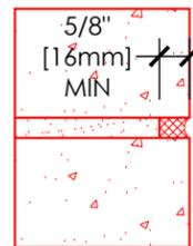
REMOVE ALL DUST AND DEBRIS FROM THE JOINT. APPLY A 1/2" [13mm] BEAD OF SEALANT IN THE JOINT
